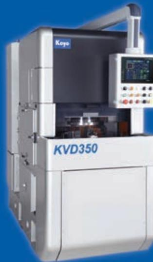
Koyo's KVD-350 is a vertical-spindle type double-disc surface grinder that is ideal for high production precision grinding. Benefits include CBN capability, reduced thermal distortion, reduced accumulation of sludge, easy operation and increased grinding capacity. Replace wheel and dresser from machine side and save space due to reduced footprint. High rigidity of grinding wheel spindle and high speed loading unit also contribute to superior performance.
